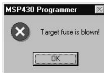
Figure 2–3. Communication Error Box for Blown Fuse
